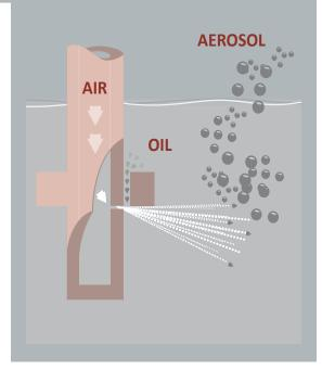
Figure 1: Aerosol generation by Laskin nozzle
