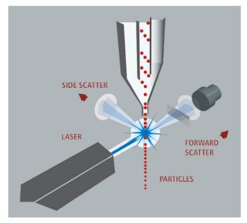
Figure 4: Principles of particle detection
